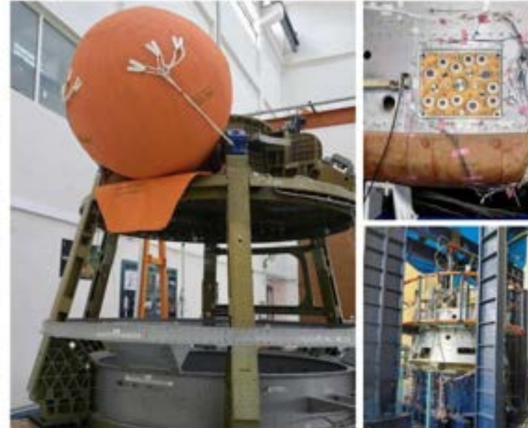
Step-by-step: (Clockwise from left) The crew module uprighting system, the service module connect disconnect system, and the apex cover that underwent testing. ISRO
