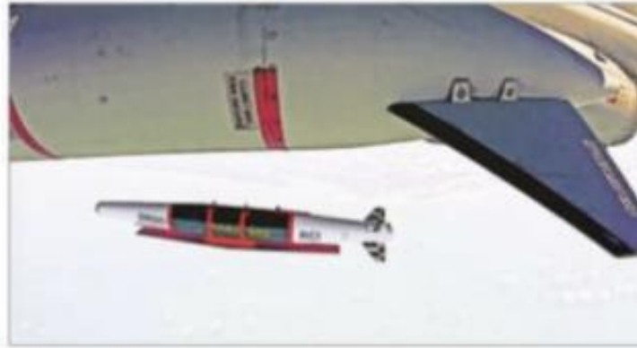
TARA is India's first indigenous glide weapon system to convert unguided warheads into precision guided missiles. X/@DRDO_INDIA
