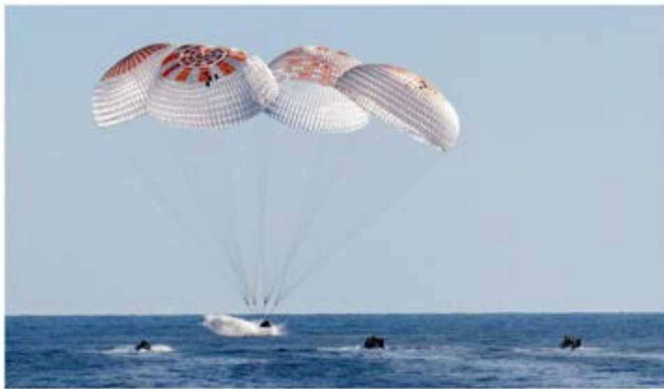
In the lower atmosphere, a returning capsule can still reach hundreds of kilometers per hour, far too fast for a safe landing, so the parachute has to be deployed to reduce the velocity for a soft landing in the sea. PH
